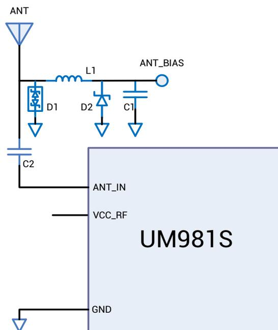
Figure 3-2 UM981S External Antenna Feed Reference Circuit
